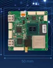
An advanced multi-stream H.264/5 codec, Jupiter-Al integrates a powerful onboard accelerator that enables highly efficient Al features such as detection, classification and tracking and other customer Al processes, with compact form factor and low power consumption for extended professional and tactical operations. Ultra-low latency enables streaming over wired and wireless networks with forward error correction (FEC) support.
