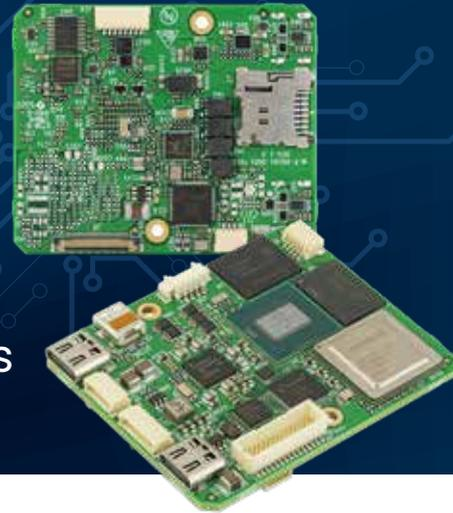
A high-end multi-channel h.264/5 codec, Jupiter SB is integrated with an onboard AI accelerator that enables highly accurate AI-powered detection and tracking capabilities and other customer AI processes.
