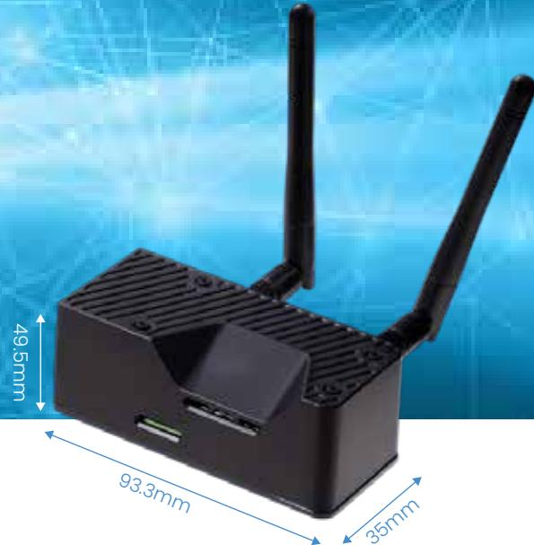
Ultra miniature and low-power H.264/H.265 multi-channel encoder/recorder, streaming real-time, high-end video over cellular and Ethernet networks.
